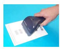
Touch™ Light readers scan barcodes on contact. All models have a hardwar trigger button which by default must be pressed to read a code. After configuring the reader interface type, the software trigger parameter (available in this manual) car be selected so that the reader operates like a model without trigger.
