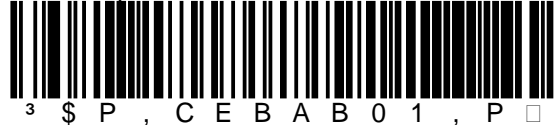
UPC E Expand to UPC A = Enable
