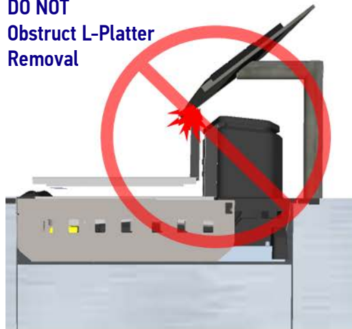
Figure 16. Vertical Clearance - Obstructions
