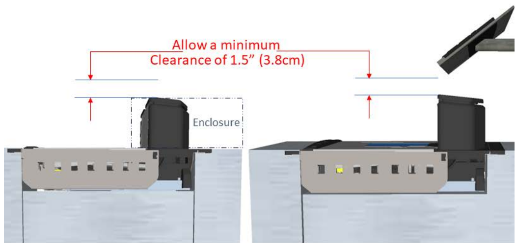
Figure 17. Vertical Clearance - Minimum Clearance
