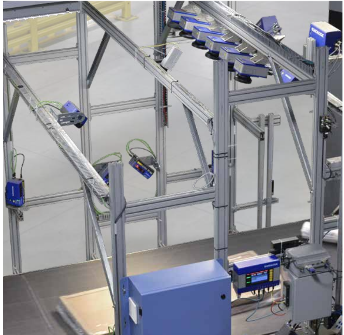
Mass Flow Detection of items on a conveyor
