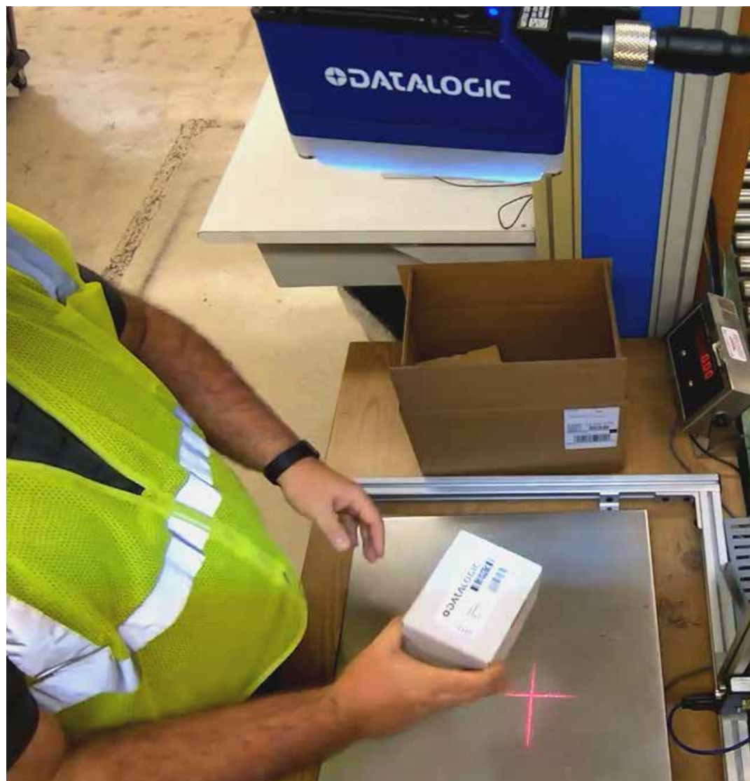
Hands-free scanning captures data as items are moved through the field of view. No need to pickup a handheld device.
