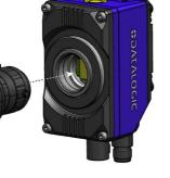
5. Mount the lens cover onto the base cover.
