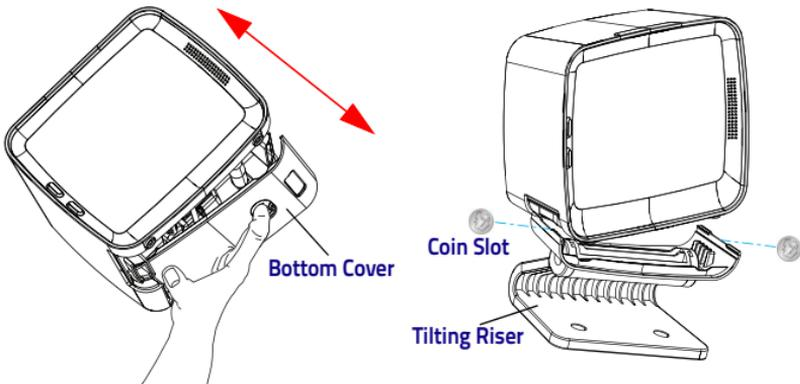
When removing the Tilting Riser, note that the snaps on the riser may be tight. If necessary, use a coin or other flat tool in the provided slots (as shown above) to separate the snaps and release the riser.
