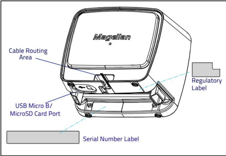
Figure 3. Scanner Features - Bottom View
