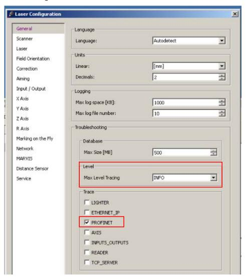
Each command that the PLC sends to the laser marker is recorded in detail in the Troubleshooting database, which can be opened as shown:
