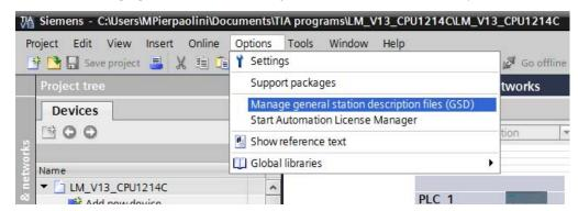
Now follow the steps in order to install the GSDML file, indicating the filepath of the GSDML file on the PC where TIA is running.
