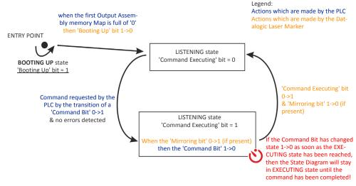
As soon as the connection is established, the State diagram is positioned at its Entry Point: the protocol will not accept any command from the PLC before receiving an Output Assembly Memory Map fully made of '0'. Until this condition is fulfilled, the Laser State Diagram will remain in BOOTING UP state and the 'Booting Up' bit=1 (the 'Booting Up' bit is bit 7 address 3 of the Input Assembly Memory Map).
