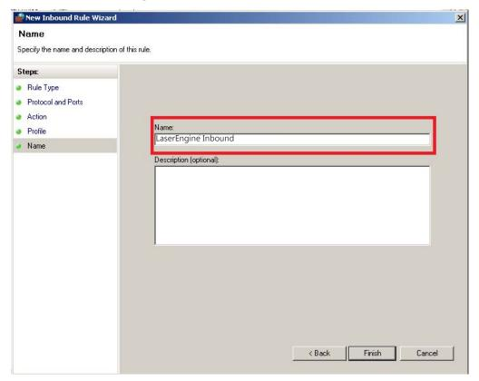
8. Now the Outbound rule must be set, making sure that all connection would be allowed also in an Output direction. Basically, the procedure must be repeated from point 2 to point 7, selecting 'Outbound Rules' at point 2 of the procedure. Once this is done, the created input and output rules will be seen along with all the other firewall rules.
