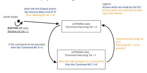
As soon as the connection is established, the State diagram is positioned at its Entry Point: the protocol will not accept any command from the PLC before receiving an Output Assembly Memory Map fully made of '0'. Until this condition is fulfilled, the Laser State Diagram will remain in BOOTING UP state and the 'Booting Up' bit=1 (the 'Booting Up' bit is bit 7 address 3 of the Input Assembly Memory Map).
