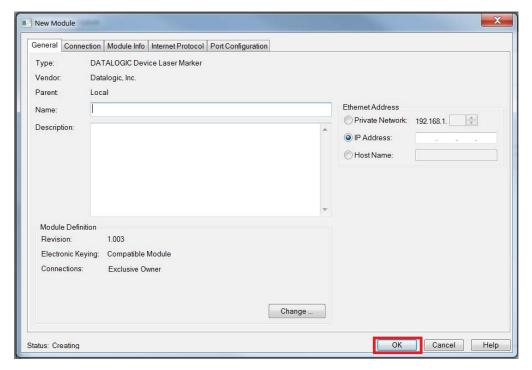
During the rest of this document, references will be made to a module called 'AREX': if the user decides to type 'AREX' inside the Name field and the IP Address entered is correct, this is what will be found as Ethernet connections inside the Studio 5000 project:
