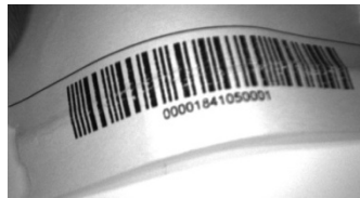
Figure 26 - Barcode Printed on Curved Surface Readable by Matrix 300N in spite of Image Optical Distortion
