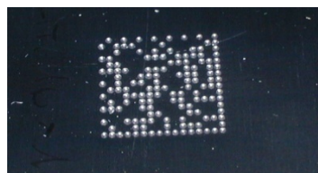
Figure 29 - Directly Marked Dot Matrix Code Characterized by Outstanding Separation Distance between Adjacent Code Elements
