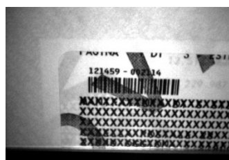
Figure 25 - Overprinted Barcode Readable by Matrix 320 2mp also Through the Envelope Window Film
