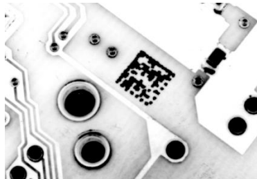
Figure 31 - Data Matrix Code Directly Marked on PCB Surface by Using Laser Etching Technology
