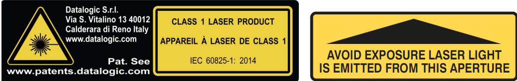
Example Laser Warning Labels for Matrix 320 2mp C-Mount models with LTM x2x-xxx DOE illuminator
