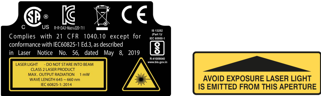
Example Laser Warning Labels for Matrix 320 2mp Liquid Lens models
