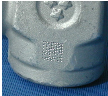
Figure 27 - Dot Matrix Code Directly Marked on Metal Surface by Using Dot Peening Technology
