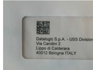
Figure 22 - Address Coded in Data Matrix Symbology for Automated Mail Processing
