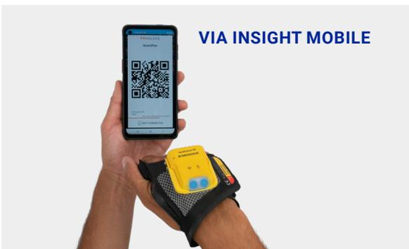
Open the app symbol "Insight Mobile" on the mobile device and scan the Pairing Barcode. To download the app and configure the device, register at <https://www.datalogic.com/handscanner/config>.
