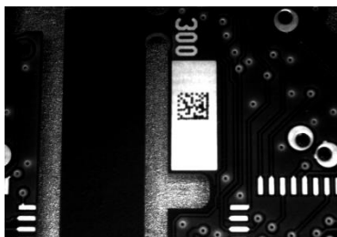
Figure 24. Dot Matrix Code Directly Marked on PCB Copper Pad by Using Ink-Jet Technology
