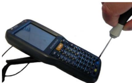
\* Always use a torx screwdriver to prevent screw damage.
