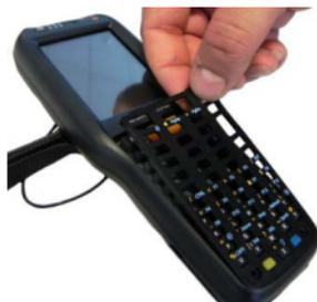
2. Insert the terminal emulation overlay (first the upper side). Fix the overlay with the screwdriver:
