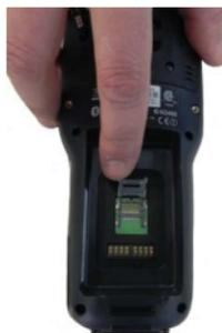
4. Insert the microSD card with the written part upward:
