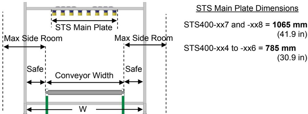
The **Safe** clearance between the frame and the conveyor sides has to be chosen according to the **Maximum Side Room** available. It is suggested to always keep at least of 200 mm of **Safe** clearance.
