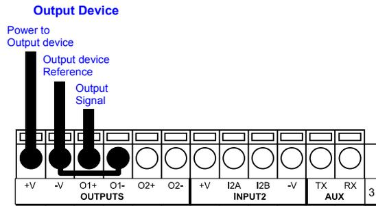
Figure 18 - Open Collector Output Using STS400™ Power
