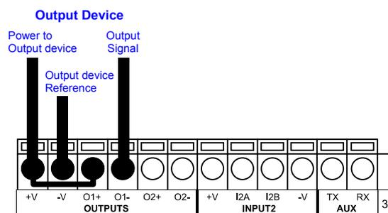
Figure 17 - Open Emitter Output Using STS400™ Power
