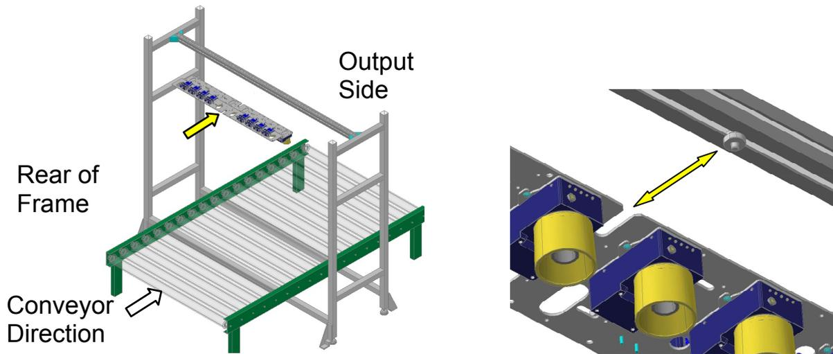
Slide the main plate slot between the plate support assembly and the supporting profile until it reaches the end.
