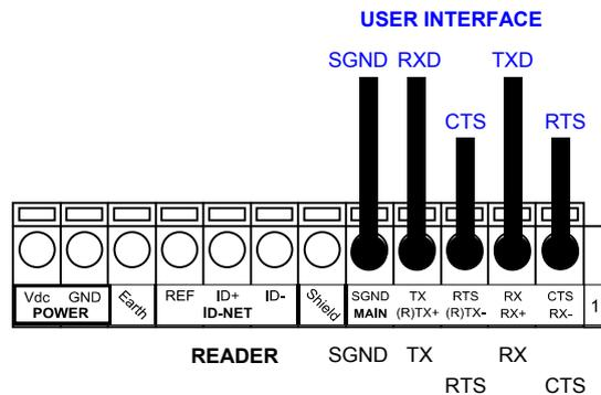
Figure 7 – RS232 Main Interface Connections Using Hardware Handshaking
