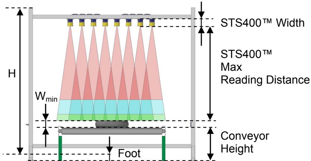
The STS400™ Maximum Reading distance is considered starting from the reader window surface to the maximum reading point:
