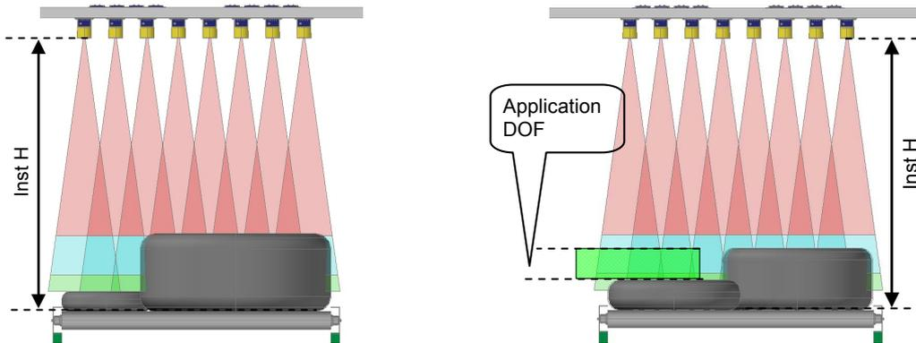
In the figure on the right, the STS400™ nominal DOF is perfectly overlapped and centered on the application DOF.
