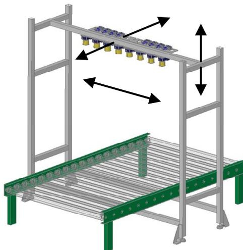
In this sample frame the STS400™ can be moved up-down, backward-forward, and left-right:
