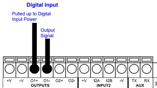
Figure 19 - Output Connected to External Digital NPN Input
