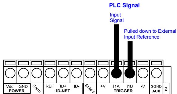
Figure 15 - External Trigger Connected to PLC
