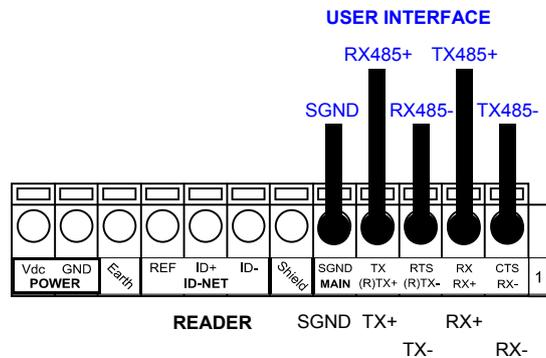
Figure 9 - RS485 Full-duplex Connections
