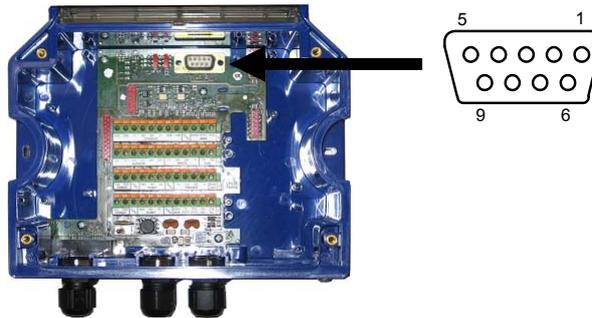
Figure 11 - 9-pin female connector
