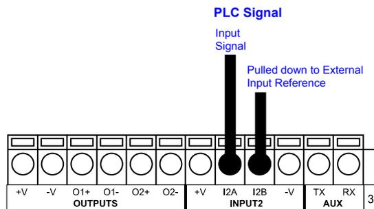
Figure 16 - Input 2 Connected to PLC
