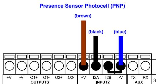
Figure 14 – Presence Sensor Connected to Input 2
