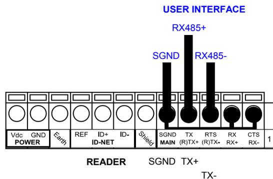
Figure 10 - RS485 Full-duplex Connections using Only TX Signals
