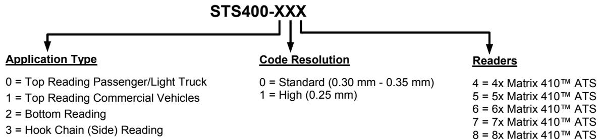
Single Matrix 410™ ATS-xxx models are used as stand alone readers having the same characteristics as the relative application type STS400™ models. They are also used as replacement readers for the relative STS400™ stations.
