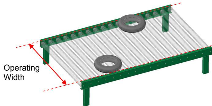
**Maximum Application FOV:** This data is the maximum reading width where a barcode can be found by the STS400™.
