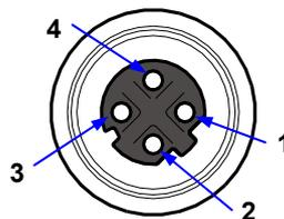
Figure 6 - M12 D-Coded Female Ethernet Network Connector
