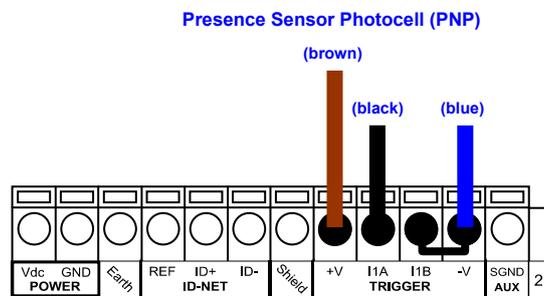
Figure 13 – Presence Sensor Connected to External Trigger
