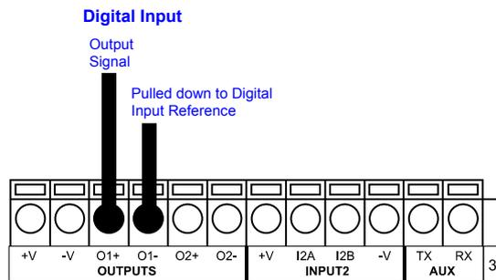
Figure 20 - Output Connected to External Digital PNP Input
