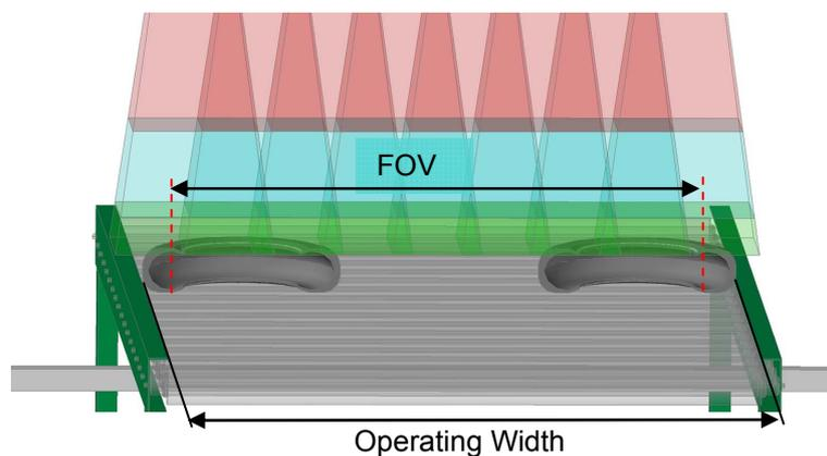
The figure above shows a sectional view of the tires in order to better understand the difference between the Maximum Application FOV and the Conveyor Operating Width.
