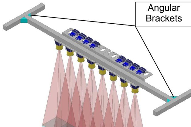
Once the frame has been fully mounted, the STS400™ can be mechanically mounted.
