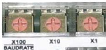
Figure 12 – Address Selection Switches
