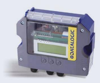
SC4000 is an industrial controller designed for high speed data collection in an ID-NET™ network of Datalogic Automation's 1D/2D code readers. SC4000 offers high communication performance and connectivity to the most common fieldbus systems by means of a complete range of optional modules.
