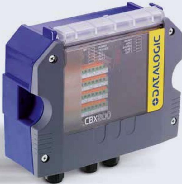
CBX800 is an industrial gateway allowing connection of devices equipped with a standard RS232 communication interface to the most common fieldbus systems, by means of a complete range of optional modules, and to ID-NET™ high speed communication network. CBX800 allows, with the same model, flexible interfacing of several devices (e.g. Datalogic Automation's 6K and 8K series, Hand Held Readers) to different networks.
