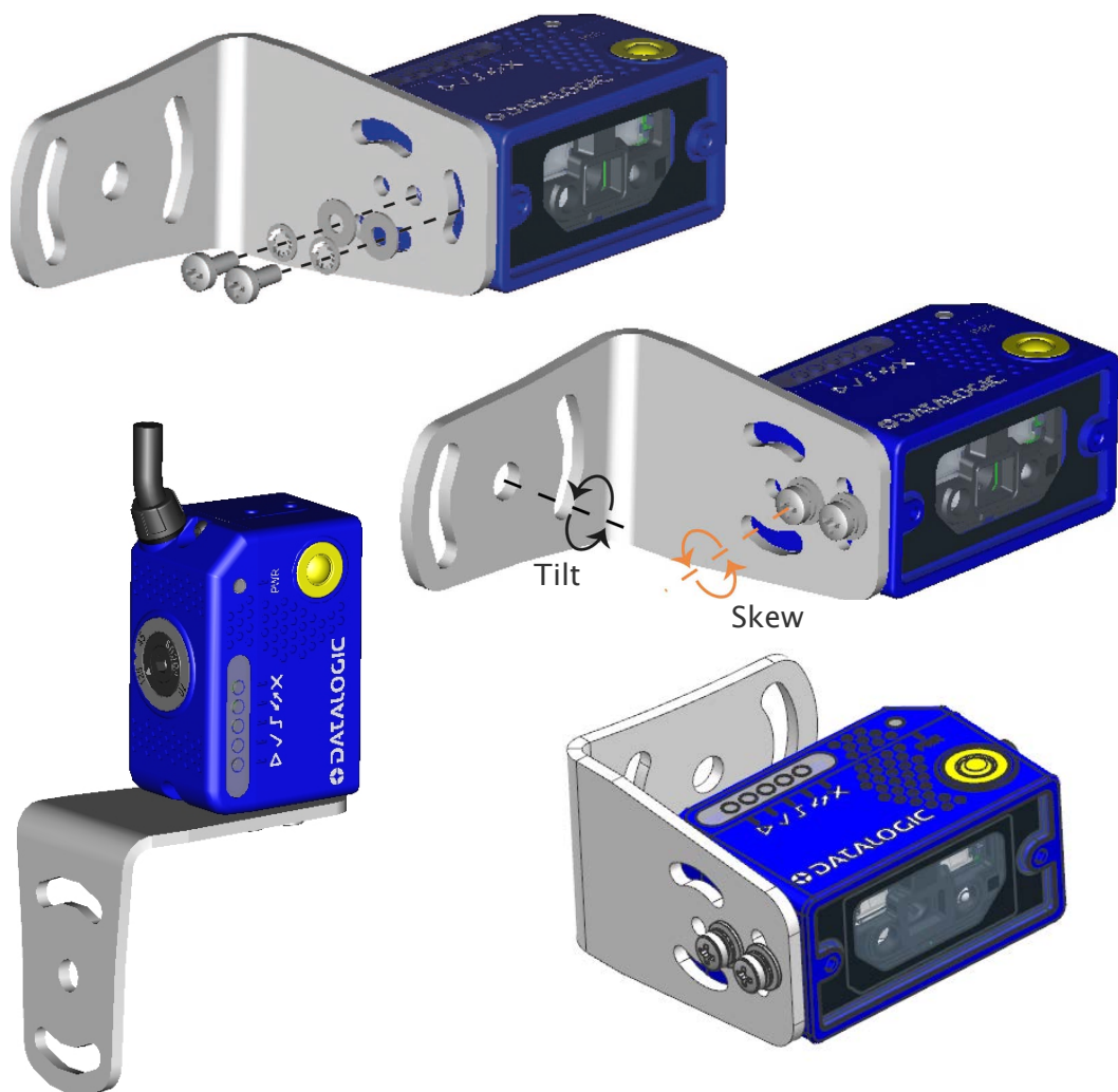
Figure 36. Side Mounting Positions for USB Models
