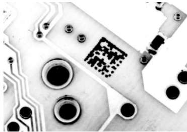
Figure 25. Data Matrix Code Directly Marked on PCB Surface by Using Laser Etching Technology
