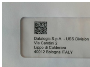
Figure 20. Address Coded in Data Matrix Symbology for Automated Mail Processing
