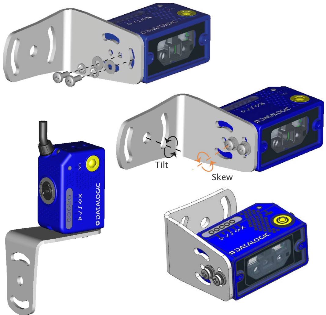
Figure 36. Side Mounting Positions for USB Models
