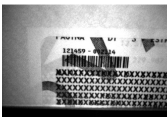
Figure 22. Overprinted Barcode Readable by Matrix 120 also Through the Envelope Window Film
